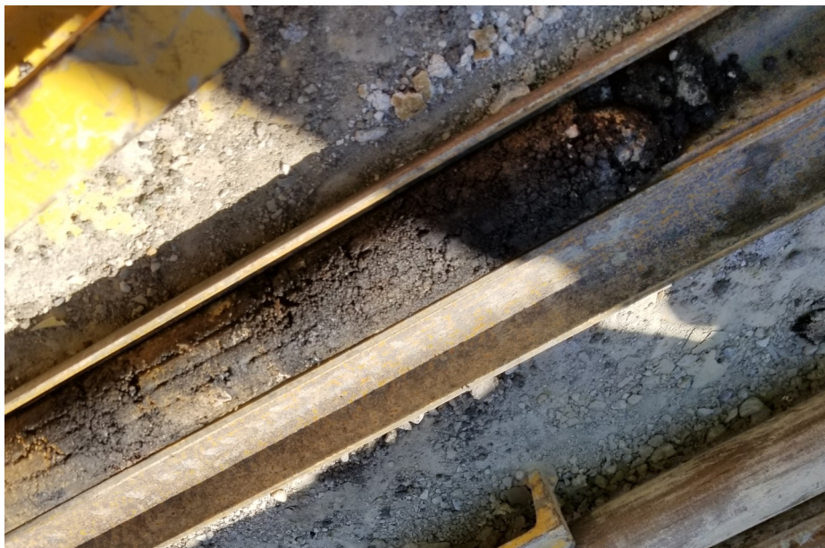
Photo 1 - Shallow black fill layer from 0.05 to 0.96 mbgs at MW-1
