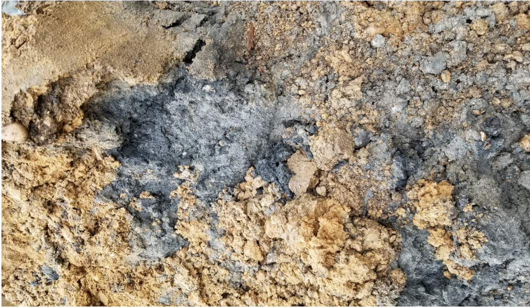
Photo 9 - Grey stained sand layer from TH-2A
