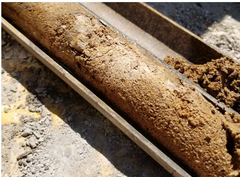
Photo 2 - Brown sand layer from 0.96 to 1.52 mbgs at MW-1
