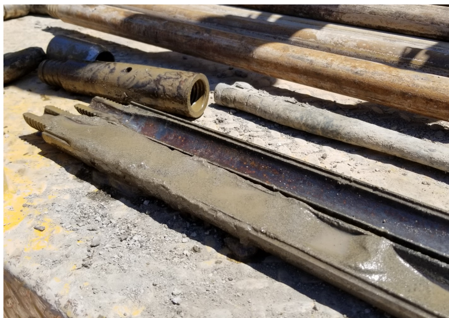
Photo 4 - Grey stained sand layer from 2.13 to 2.90 mbgs in MW-2
