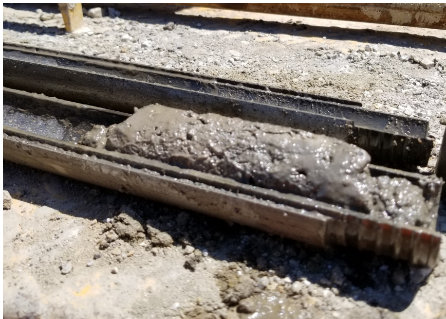
Photo 3 - Grey stained sand and stones layer from 1.37 to 2.13 mbgs in MW-2
