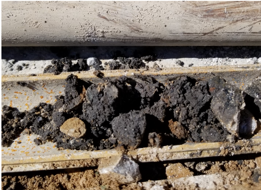
Photo 5 - Black fill layer from 0.05 to 1.37 mbgs in MW-3
