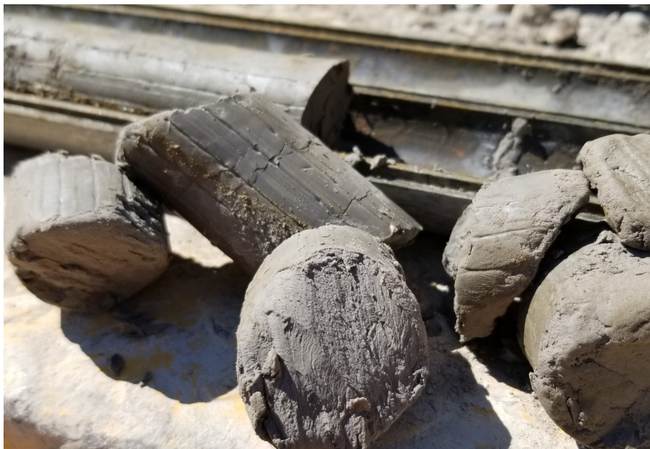
Photo 6 - Grey clay layer from 1.37 to 2.13 mbgs in MW-3
