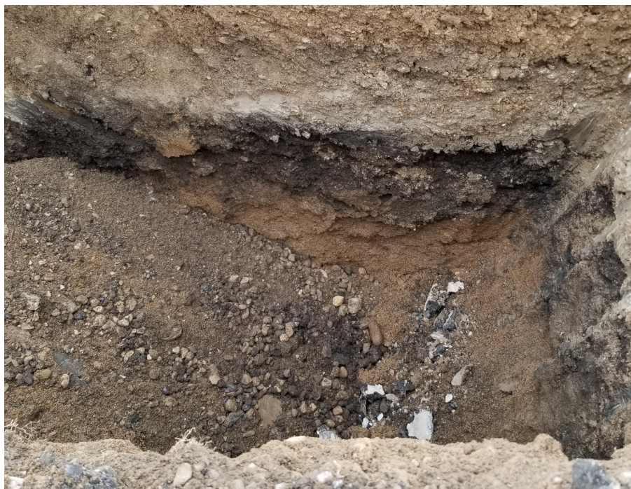
Photo 8 - View of TH, showing black fill layer between brown gravel fill and brown sand layer.
