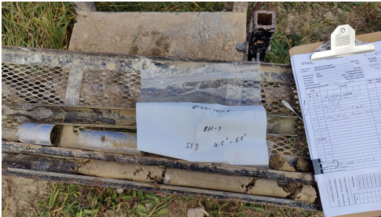
Picture 18: Soil Sample Retrieved in the SPT Spoon.
