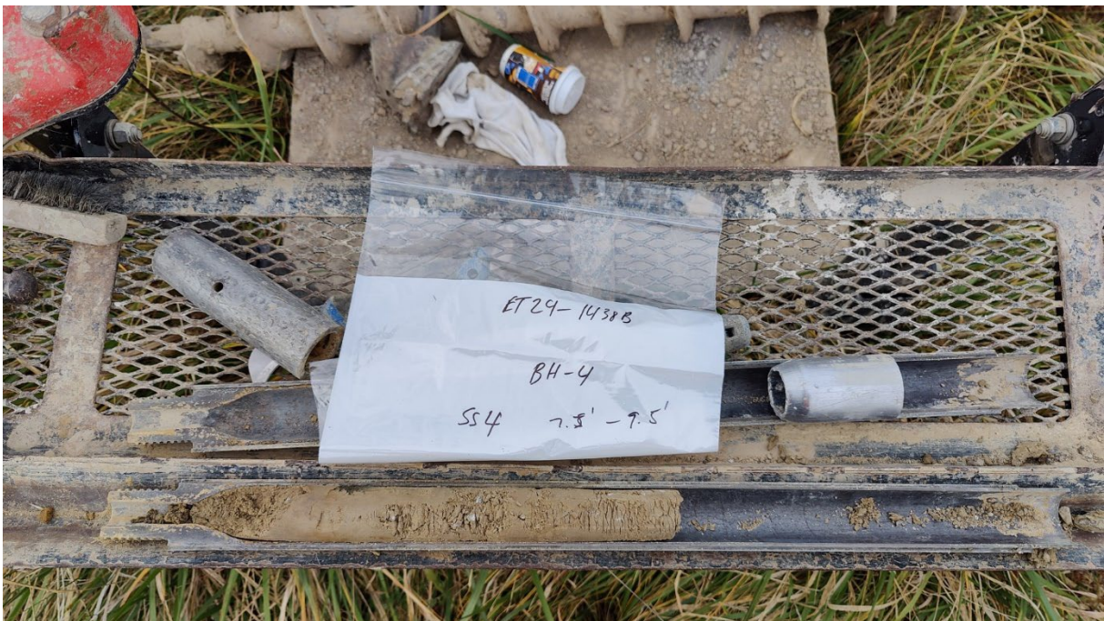
Photograph 16: Soil Sample Retrieved in the SPT Spoon.
