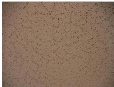
Photo 1: Non-asbestos 24" x 48" lay-in acoustic ceiling tile with a random fleck and pinhole pattern.
