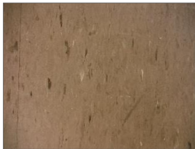
Photo 3: Non-asbestos 12" x 12" brown vinyl floor tile with flecks.
