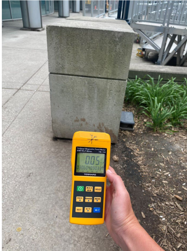
Figure 13 & 14: A.C. magnetic field readings taken in future outdoor play area.
