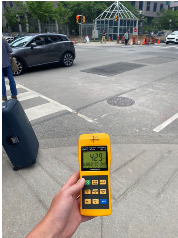
Figure 3 & 4: A.C. magnetic field readings taken outside Hydro One high voltage switch yard.
