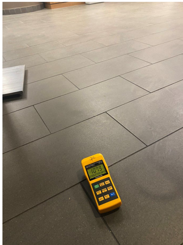
Figure 12 A.C. magnetic field readings taken at floor level above main electrical room.
