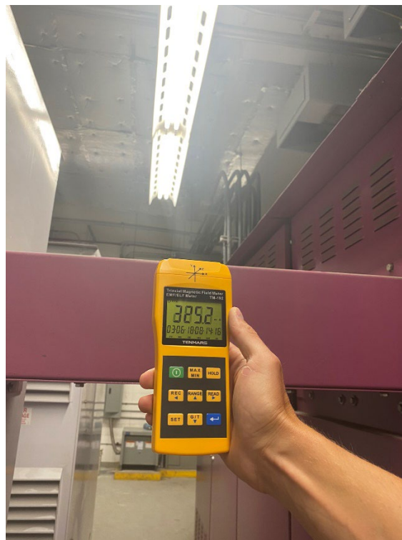
Figure 10: A.C. magnetic field readings taken beside main transformer located in main electrical room.
