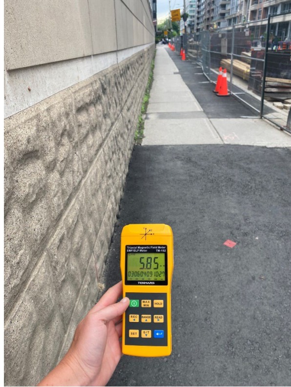
Figure 3 & 4: A.C. magnetic field readings taken outside Hydro One high voltage switch yard.
