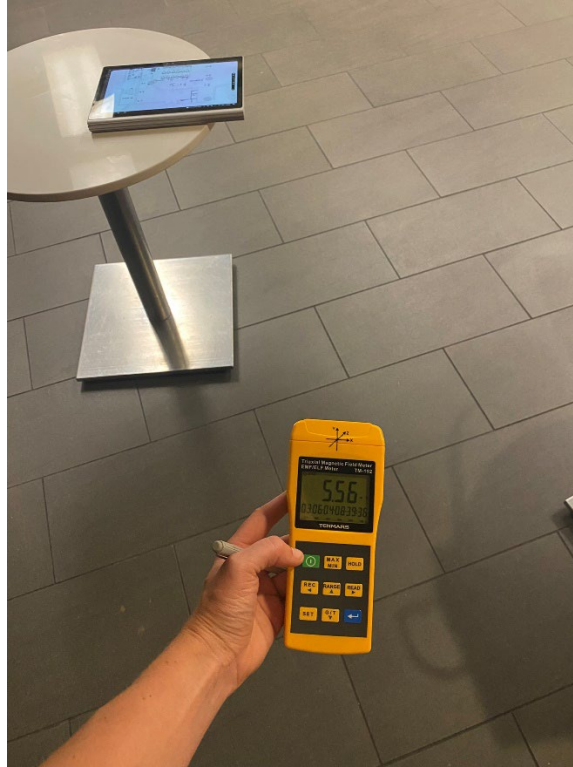
Figure 11 A.C. magnetic field readings taken at 3ft above main electrical room
