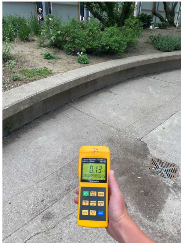
Figure 13 & 14: A.C. magnetic field readings taken in future outdoor play area.
