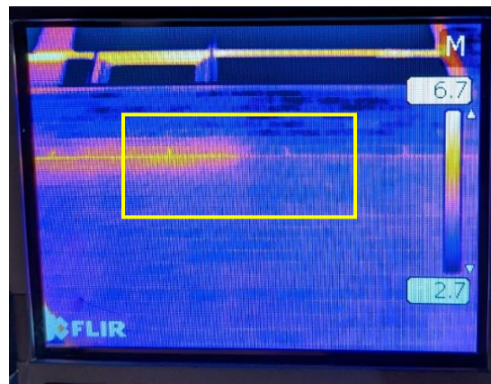
Image 4 – Thermal anomaly beneath window
