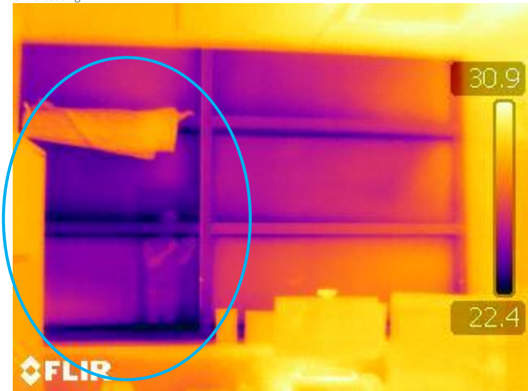
Photograph No. 20 Thermal anomalies at window mullions on left side, from the interior.
