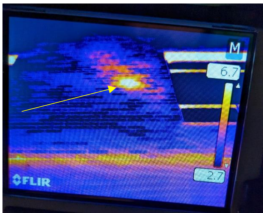
Image 3 – Thermal anomaly to left of window
