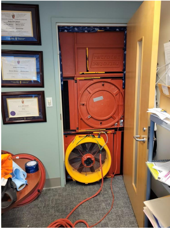
Photograph No. 41 Blower door set up, office 1EW421.
