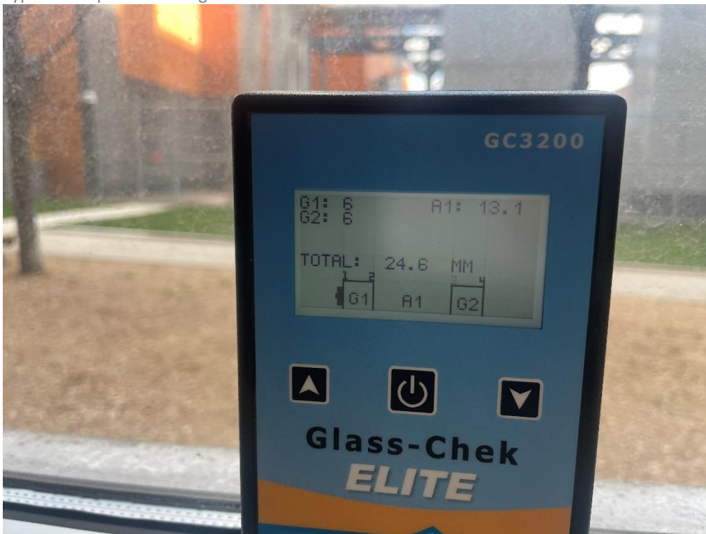
Photograph No. 6 IGU thickness reading.
