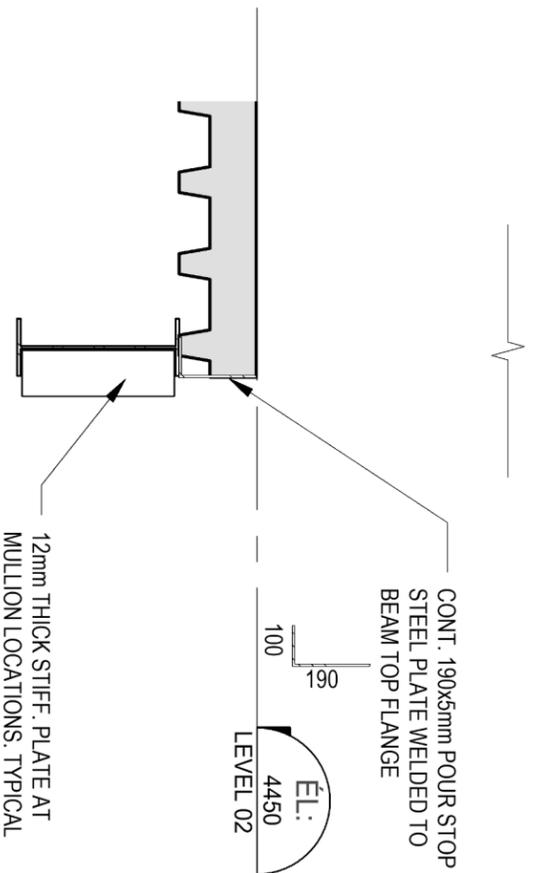
CONT. 190x5mm POUR STOP STEEL PLATE WELDED TO BEAM TOP FLANGE
