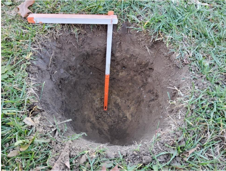
Image 5: Typical undisturbed test pit profile (surface A-horizon) in the northwest of the project area.
