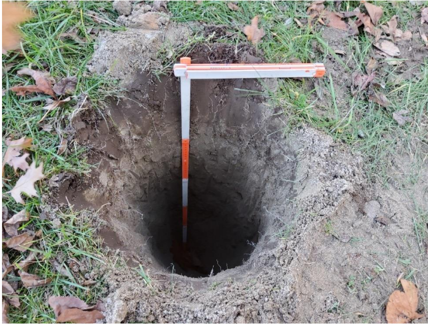
Image 7: Typical disturbed test pit profile in the southeast of the project area.
