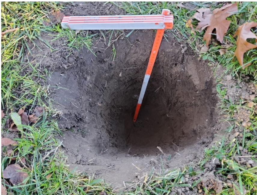
Image 6: Typical undisturbed test pit profile (buried A-horizon) in the west of the project area.
