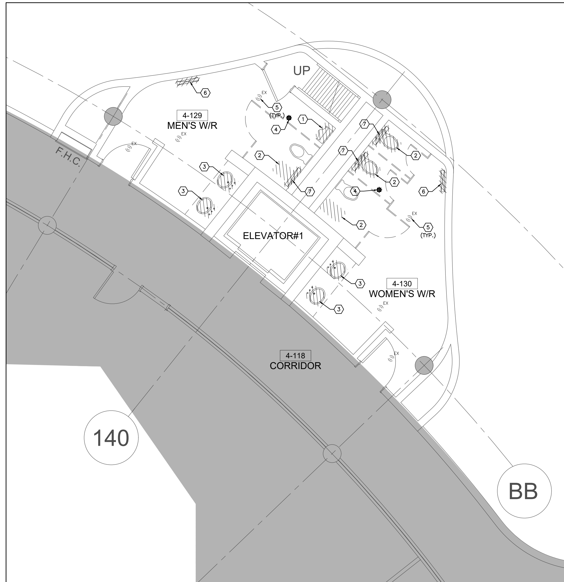
3 WASHROOMS 4-129 & 4-130 - MECHANICAL DEMOLITION PLAN SCALE: 1:50
