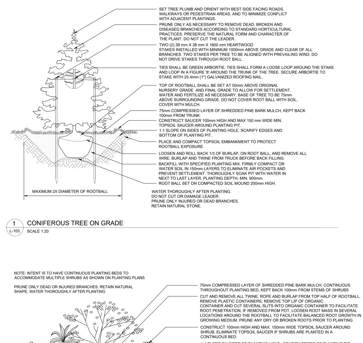
1:1 SLOPE ON SIDES OF PLANTING HOLE. SCARIFY EDGES OF PLANTING PIT. FIRMLY COMPACT OR WATER TOPSOIL IN 150mm LAYERS TO ELIMINATE AIR POCKETS AND PREVENT SETTLEMENT
