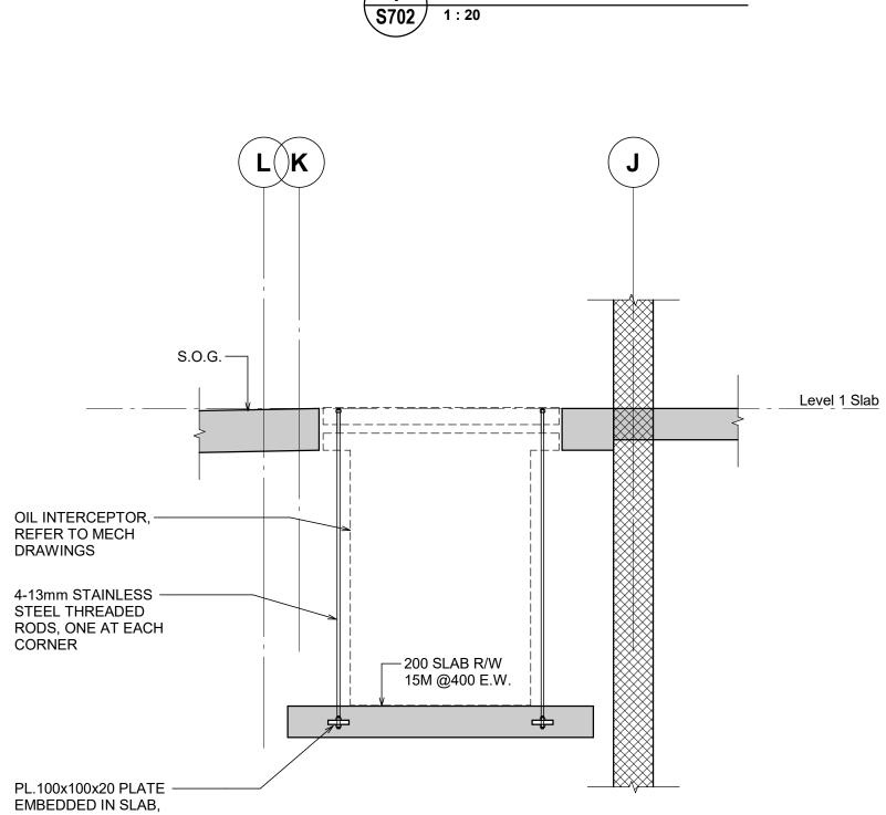
PL.100x100x20 PLATE EMBEDDED IN SLAB, FASTENED WITH NUT EACH SIDE, TYP. AT ENDS OF THREADED RODS
