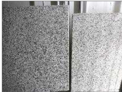
Photo 12: Non-asbestos Tectum tiles in Storage Cages (Location B-002).
