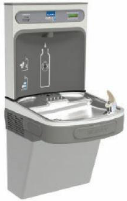
DRINKING FOUNTAIN: DF EZSDWSLK GALVANIZED STEEL WALL MOUNTED, WHEELCHAIR TYPE WATER COOLER WITH STAINLESS STEEL TOP, FRONT AND SIDE MOUNTED PUSH TO OPERATE LEVER(S), SENSOR, TOUCHLESS ACTIVATION WITH AUTO SHUT OFF BOTTLE FILLER, FLEXI-GUARD SAFETY BUBBLER, AND TRAP PACKAGE.
