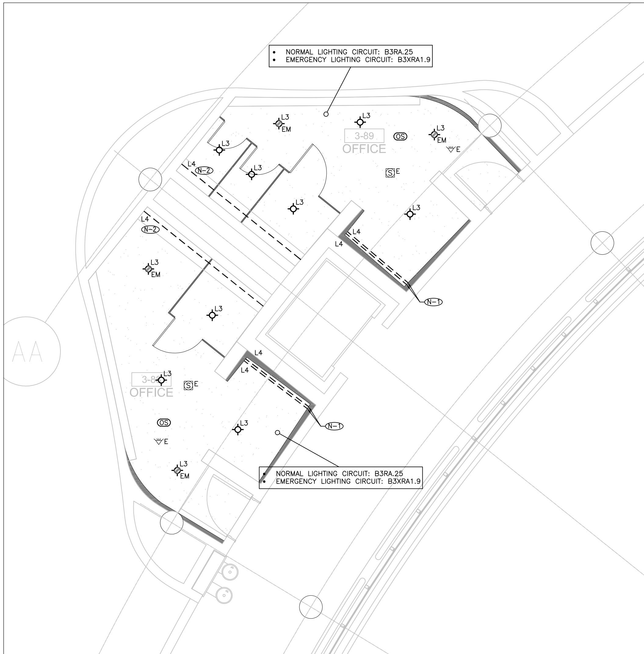
3 LEVEL 3 CEILING PLAN – W/R'S 3–88 & 3–89 E-3.5 SCALE: 1:50
