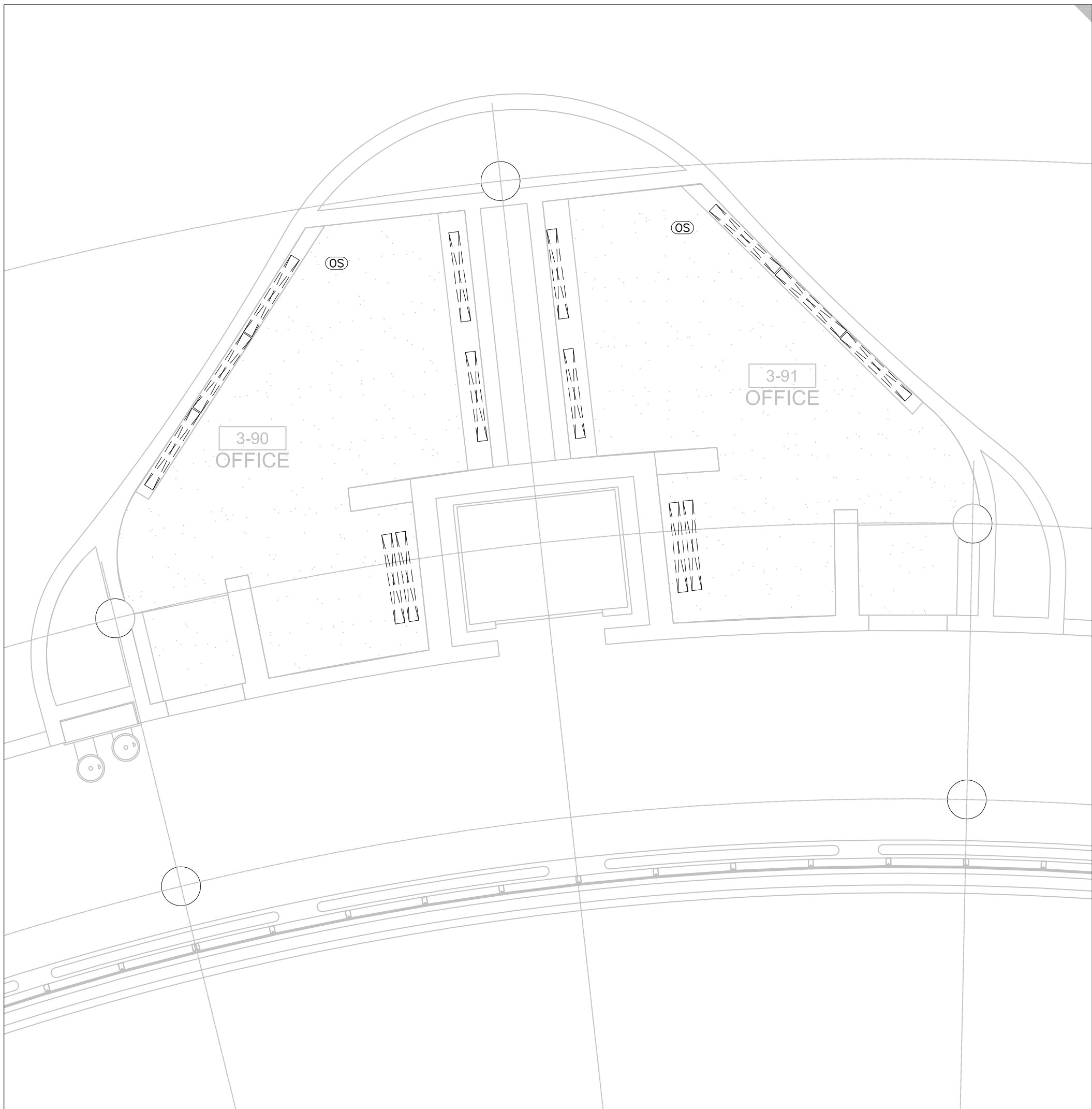
2 LEVEL 3 CEILING DEMOLITION – W/R'S 3-90 & 3-91 E-3.7 SCALE: 1:50
