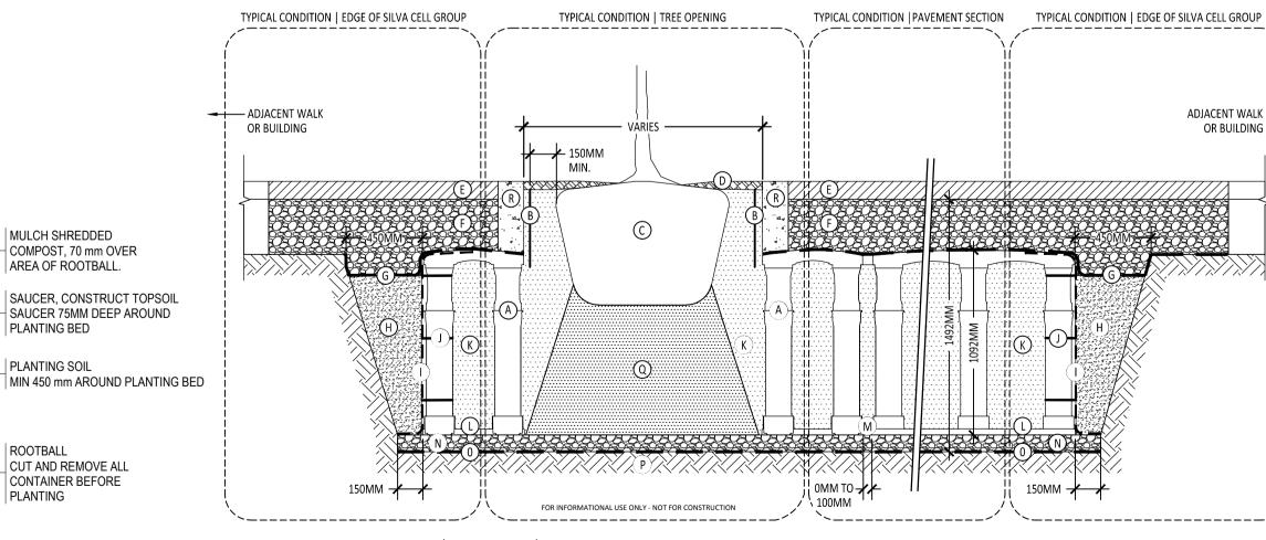
PLAZA APPLICATION | FLEXIBLE.3x | 3x SILVA CELL SYSTEM FOR PAVERS OR ASPHALT PAVING ON AGGREGATE BASE - SECTION NOT TO SCA
