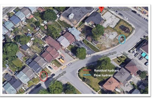
**Flow Test Measurements**
