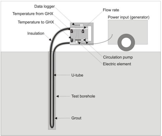
Figure 2: Thermal conductivity testing unit connected to U-tube in test borehole.
