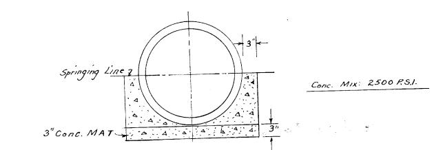
STORM SEWER TYPICAL VERTICAL SECTION
