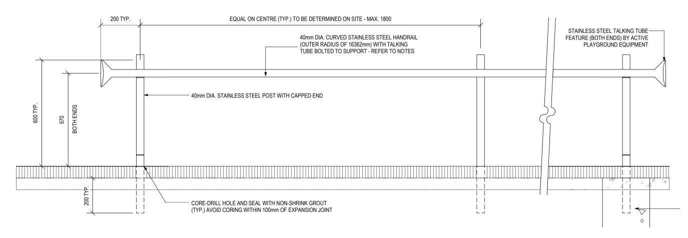
WALKING AND TALKING TUBE RAILING DETAIL 5 LD-04 scale: n.t.s.
