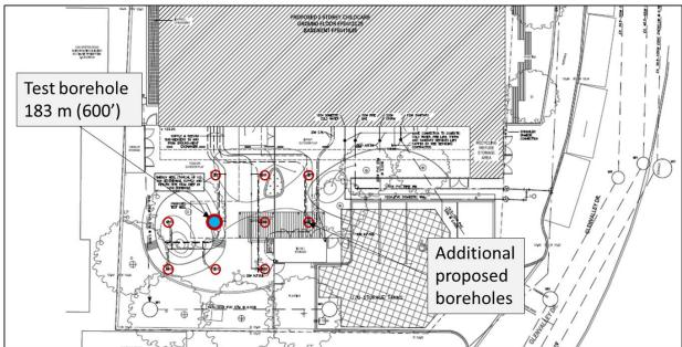
Figure 1: Borehole location and location of additional 9 proposed boreholes.
