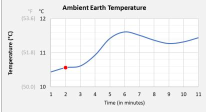
Figure 3: Based on the logged temperatures the ambient earth temperature is 10.6°C (51.0°F)
