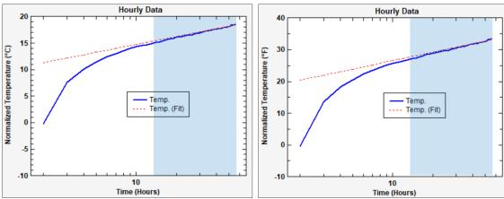
Figure 5: Graphs the fluid temperature versus the natural log of time. The slope of the line is used to calculate the average thermal conductivity of the borehole.
