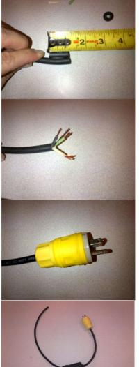
1. Remove 1" of cab tire casing & strip wires at each end
