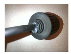
4. Using silicone seal around the cord and plug. This will help prevent water from entering the boot.
