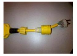
2. Disassemble the plugs end and remove only the straight blade portion. Then take a new Twistlock out of pkg and install it. The bases are interchangeable.
