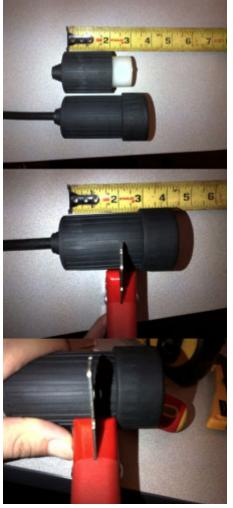
1. Boot needs to be cut back to expose the Hubbell Plug End
