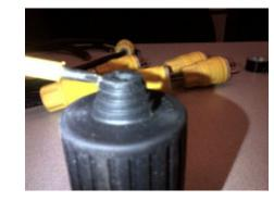
Boot Top needs to be cut. Only the Top section needs to be removed. Use a Cable cutter to get best results
