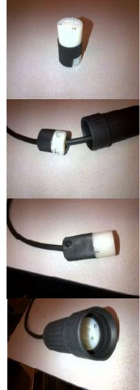
4. Disassemble the Hubbell end
