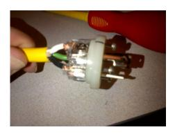
3. Once the new Twist Lock has been installed use a permanent marker to place inspection marks above the connections points to verify correct wire placement
