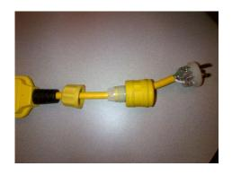
2. Disassemble the plugs end and remove only the straight blade portion. Then take a new Twistlock out of package and install it. The bases are interchangeable.
