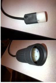
7. Slide Hubbell boot over plug pulling it over plug end under it is seated firmly at the back of boot.
