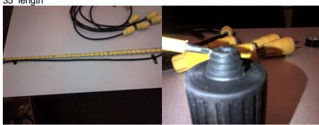
Boot Top needs to becut. Only the Top section needs to be removed. Use a Cable cutter to get best results
