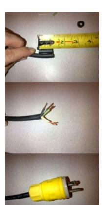
1. Remove 1" of cab tire casing & strip wires at each end
