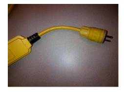
1. This is what it comes like from manufacturer. It has a straight blade wetgaurd plug which needs to be replaced with a Twist Lock wetgaurd.
