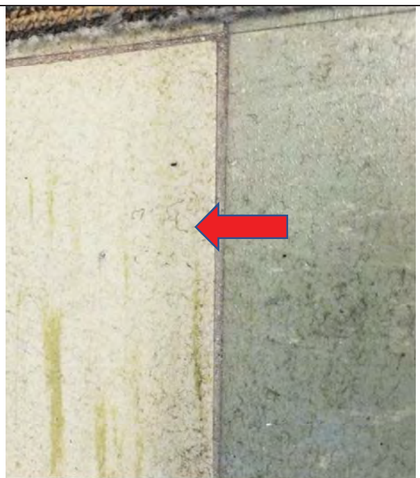
Photo 6: White with green streaks (Left tile, LEX sample 20). 2% Chrysotile.
