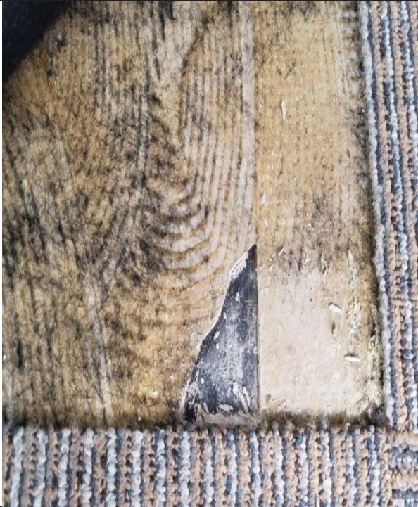
Photo 13: VFT – Brown with white streaks 9x9 (LEX sample 17). 0.5% Chrysotile.
