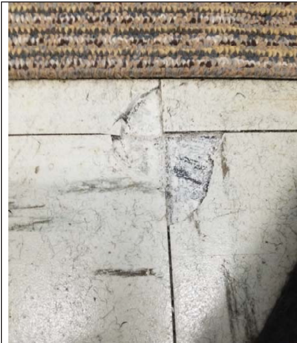
Photo 9: VFT – White with brown streaks 9x9 (LEX sample 31). 1% Chrysotile.
