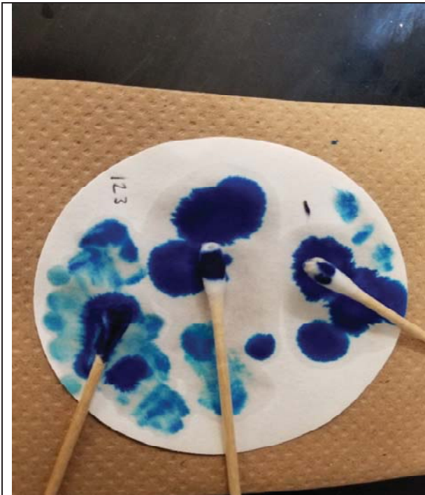
Photo 21: Representative perchlorate test results completed in room 123's fume hood. No purple precipitates detected.
