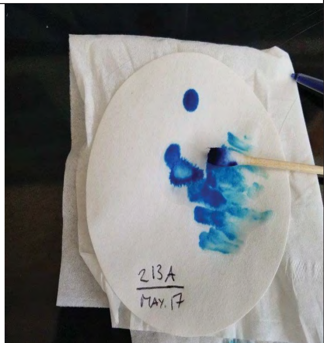
Photo 20: Representative perchlorate test result completed in room 213A's fume hood. No purple precipitates detected.
