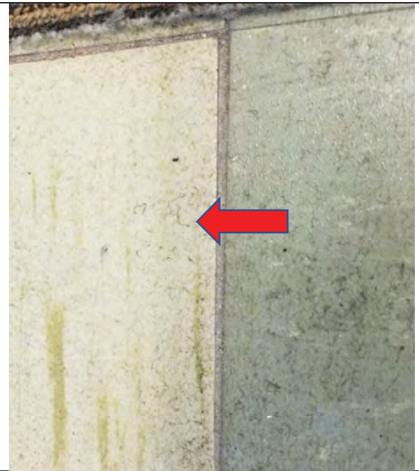
Photo 6: White with green streaks (Left tile, LEX sample 20). 2% Chrysotile.
